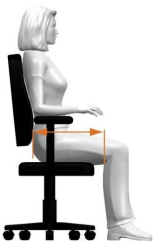
Figure 4. Seat Depth (horizontal distance between the buttock and the back of the knee)
